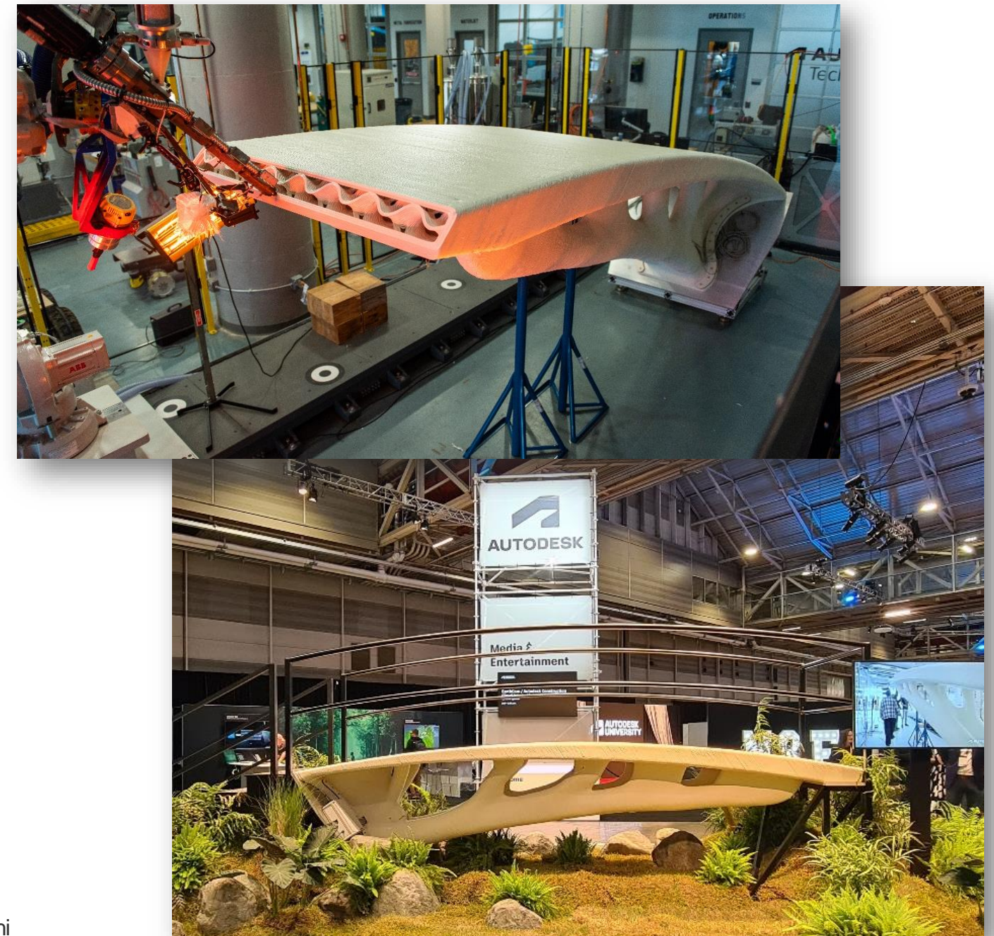
A 5m long 3D printed bridge with FGF, using recycled PETG granulates from Mitsubishi Chemical Group. Source: Autodesk
